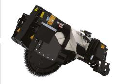
Designed for skid steer mounting, Simex RW and RWA wheel saws provide different solutions for working on hard or compact surfaces such as asphalt, concrete and rock: cutting and narrow trenches, set-section trenches, mini- and micro-trenches for fiber optic cable installation. Full protection of the wheel at any working depth guarantees maximum safety of persons and property.
