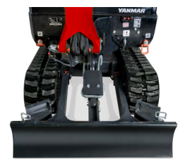
Retracted undercarriage : 980 mm
