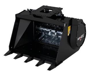
Designed to **reduce the volume of aggregates** directly on site, CBE crusher buckets with rotor system provide optimal performance when working with iron, rock, soil and deformable parts, and wet or humid materials. Ideal for crushing reinforced concrete and demolition waste. The exceptional cutting force allows any material to be crushed. The rotor with teeth is activated by high-displacement radial piston hydraulic motors in direct drive.
