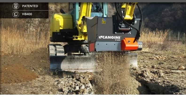
IDEAL BOTH FOR THE GRADING OF BULK MATERIALS FROM DEMOLITION OR DIGGING WORKS AND THE MIXING OF TERRAIN AND PEAT. THE SCREENING OPERATION IS CARRIED OUT BY AN HYDRAULIC SIEVE WITH ROTATING HB400 KNIVES. THE MATERIAL THICKNESS CAN VARY FROM 0 TO 20 MM (0 - 0,8 IN) AND 0 TO 35 MM (0 - 1,4 IN) WITH A STANDARD EQUIPMENT. CUSTOMERIZED SHAFTS CAN ALSO BE SUPPLIED.
