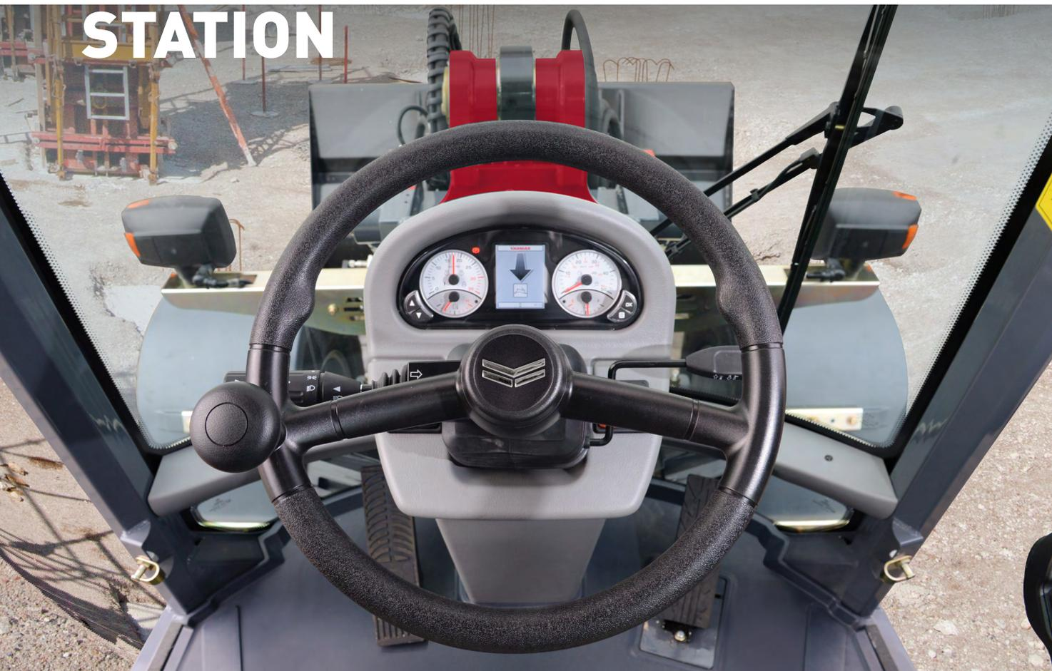
Designed with driver comfort and productivity in mind, the cabine features noise and vibration damping and is ROPS/FOPS- approved.
