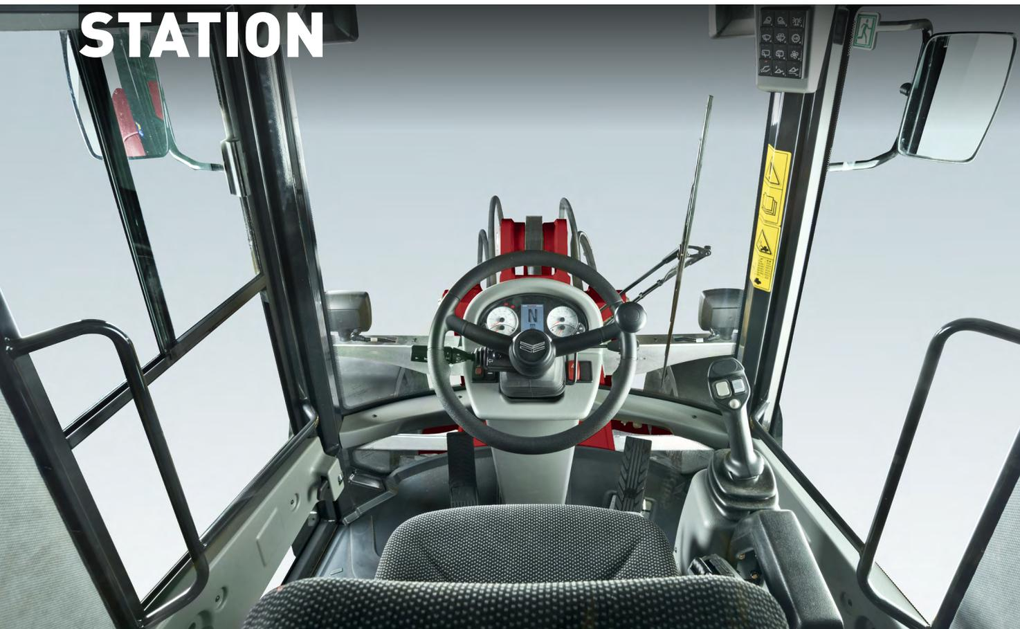
Designed with driver comfort and productivity in mind. The case feature ROPS and optional FOPS and noise and vibration damping - approved.
