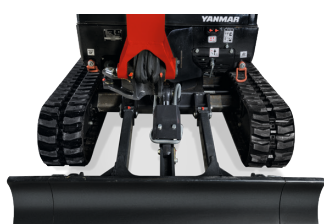
Extended undercarriage: 1170 mm
