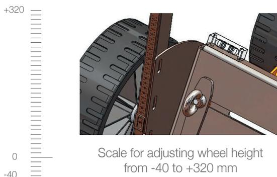
Scale for adjusting wheel height from -40 to +320 mm
